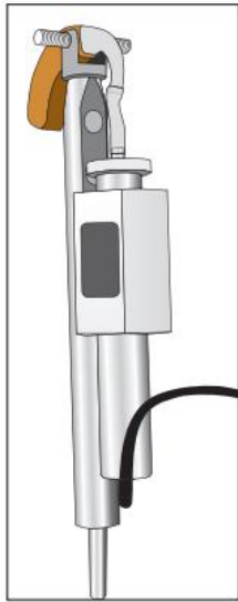
Figure 6.3.1B: BTE hearing aid positioned on Rotating Shaft and Positioning Saddle
